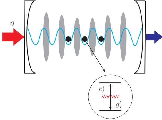
FIG. 1. (Color online) Sketch of setup:  $N_a$  ultracold spin-polarized Fermi atoms are trapped in a Fabry-Pérot cavity. A 1D classical optical-lattice potential (blue line) along the cavity axis is engineered to confine the atoms into a lattice gas. The cavity field, which couples to the atomic internal energy levels  $|e\rangle$  and  $|g\rangle$ , is pumped by a laser beam with strength  $\eta$ .
