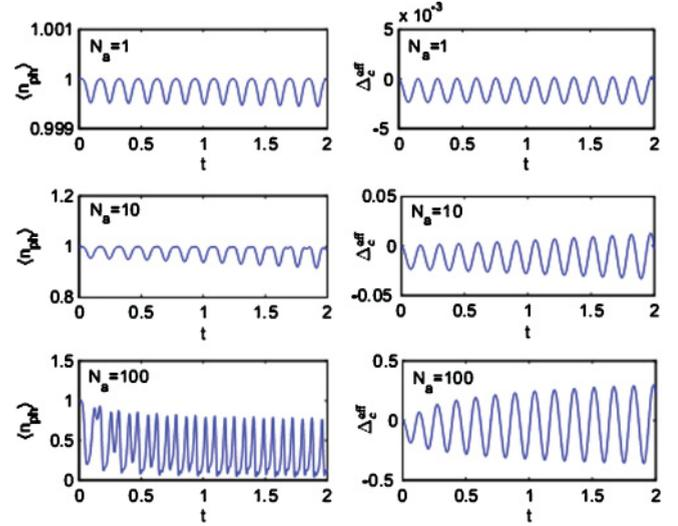
FIG. 4. Evolution of cavity photon number  $\langle \hat{n}_{\text{ph}} \rangle$  (left panels) and effective cavity detuning  $\Delta_c^{\text{eff}}$  (MHz, right panels) with times  $t$  for different atom numbers  $N_a = 1, 10, 100$ , with corresponding filling  $\nu = 0.0025, 0.025, 0.25$ , respectively. Other parameters are the same as in Fig. 2 with  $\eta/\kappa = 1$ .
