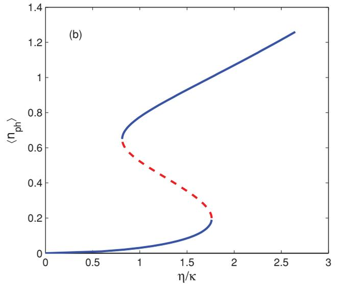
FIG. 2. (Color online) Steady-state intracavity photon number as a function of (a) pump-cavity detuning for (by increasing maxima)  $\eta/\kappa = 0.1, 0.3, 0.5, 0.7, \text{ and } 0.9$ ; (b) pumping strength for  $\Delta_c = 1.4$  MHz. Other parameters are chosen as  $t/\kappa = 0.1$ ,  $N_a = 200$ , and  $U_0 = 10$  kHz.
